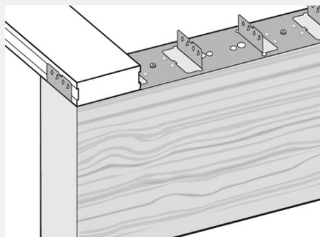
\* - Use only dome-head nails from "coil-nail" gun. Pre-drill and hand nail when within 50mm of end of board. Not our preferred fixing method.
